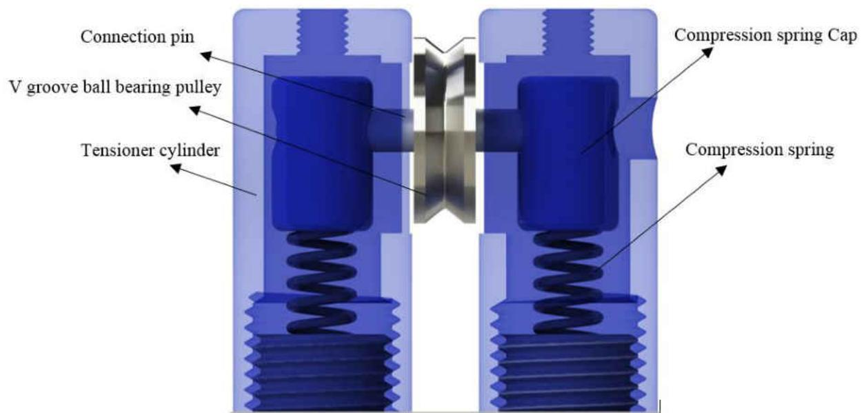
Fig. 40 CAD model of tensioner and components inside
