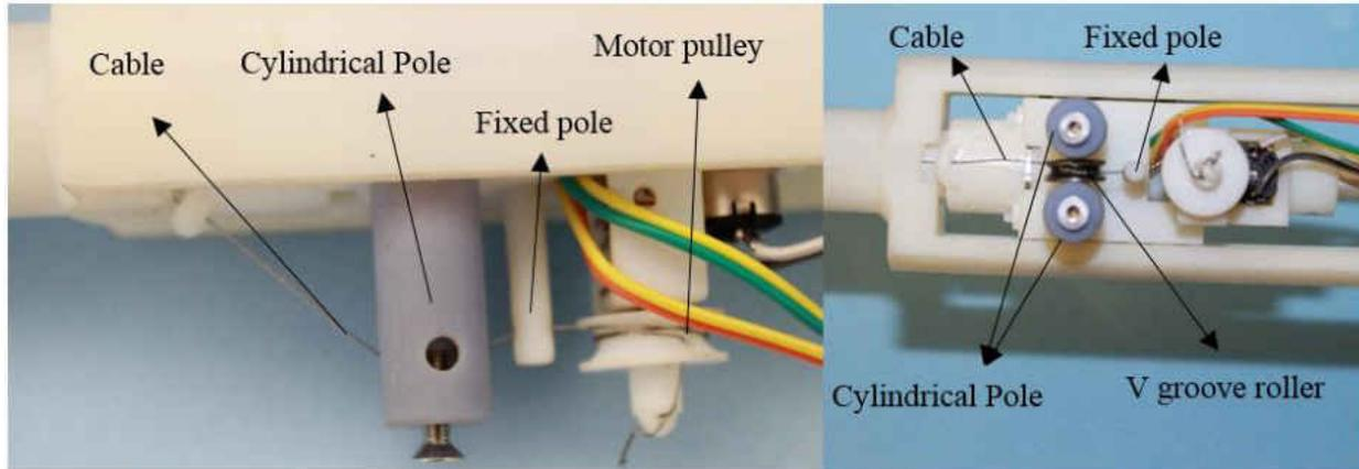
Fig. 39 Tensioner mechanism of the fingered grasper cable
