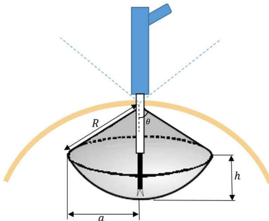
Fig. 13 Schematic of workspace of the RoboCatch
