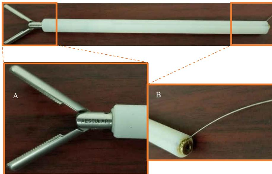
Fig. 35 Assembled grasping forceps system of RoboCatch
