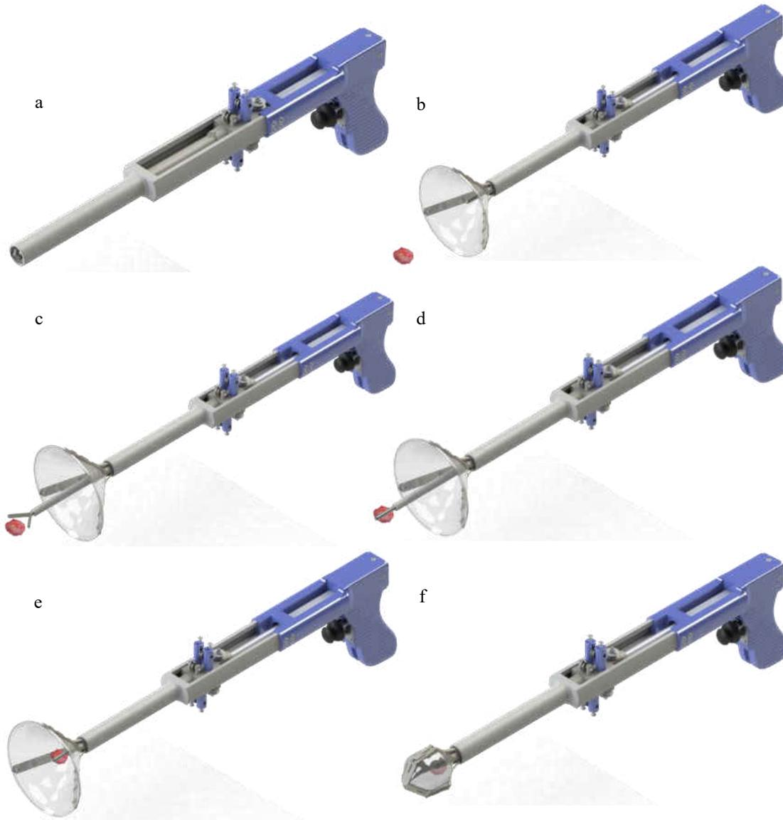
Fig. 11 Stages of specimen retrieval for the RoboCatch
