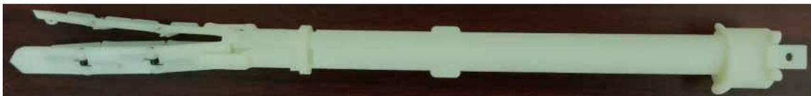
Fig. 29 Full assembly of the middle tube and the three-fingered grasper
