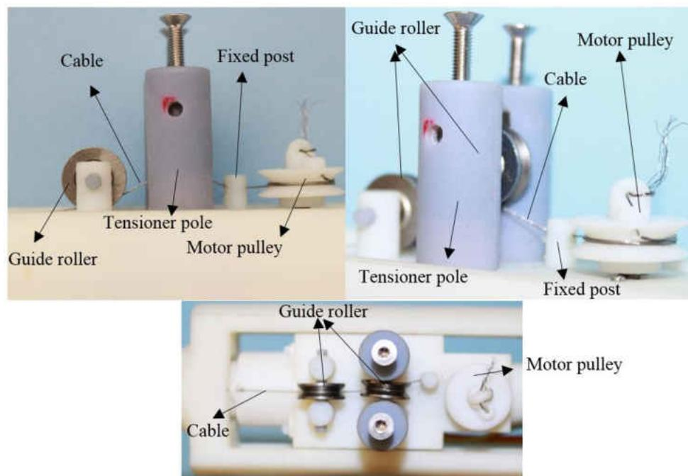
Fig. 38 Tensioner mechanism of the grasping forceps cable
