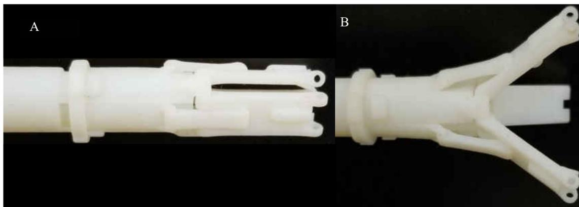
Fig. 27 Fabricated interconnected slider-crank mechanism of the RoboCatch
