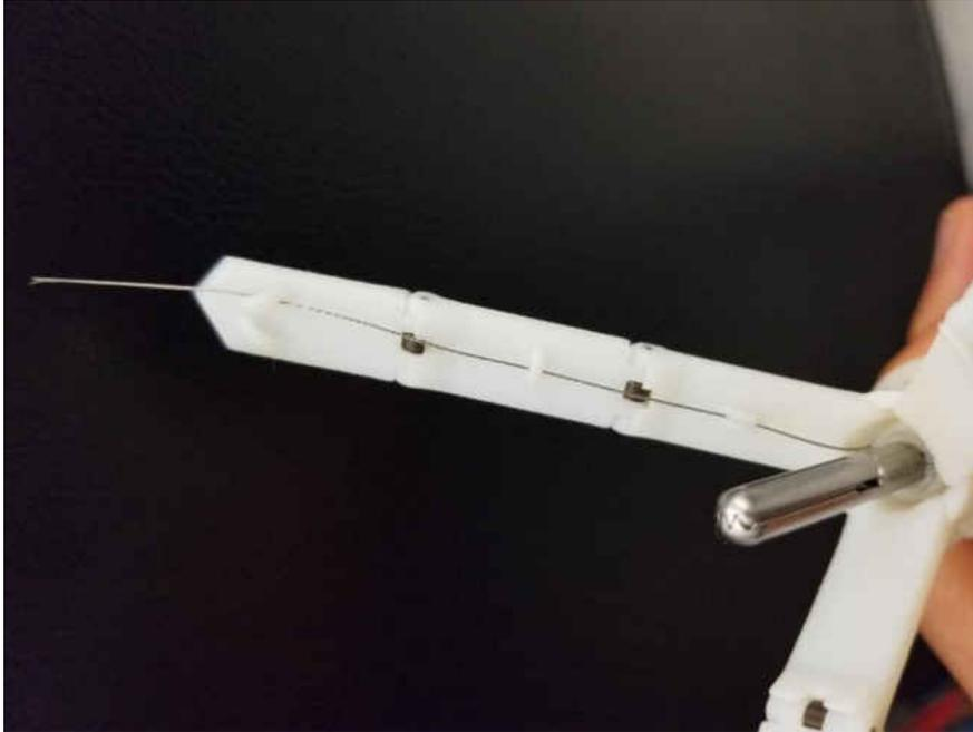
Fig. 20 Cable routing of the webbed-three fingered grasper
