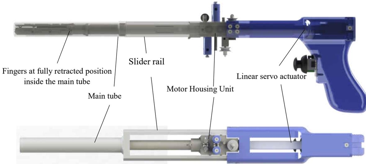
Fig. 17 Side and top view of the RoboCatch
